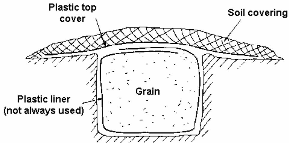
Figure 1: Cross section of underground pit storage
