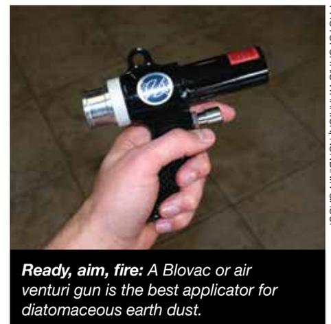
**Ready, aim, fire:** A Blovac or air venturi gun is the best applicator for diatomaceous earth dust.
